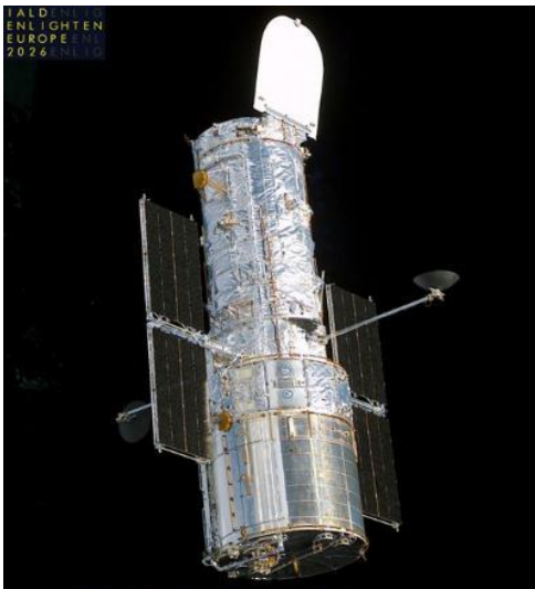
Hubble Telescope 1990 orbiting Earth Ritchey-Chrétien reflector 2.4m dia. wavelengths near IR, visible spectrum and UV Image: NASA Marshall Space Flight Center Collection (NIX MSFC-7995584), Public Domain https://commons.wikimedia.org/w/index.php?curid=1900102
