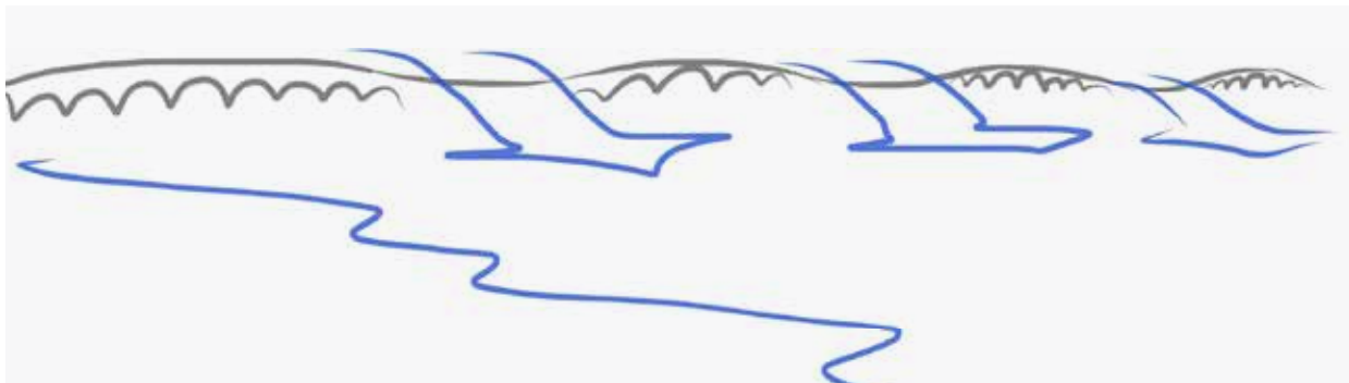
ABOVE Ian Ritchie’s iPhone digital sketch of Büyükçekmece bridge showing how flood waters flow over the bridge, a technique devised by Sinan to avoid structural damage
