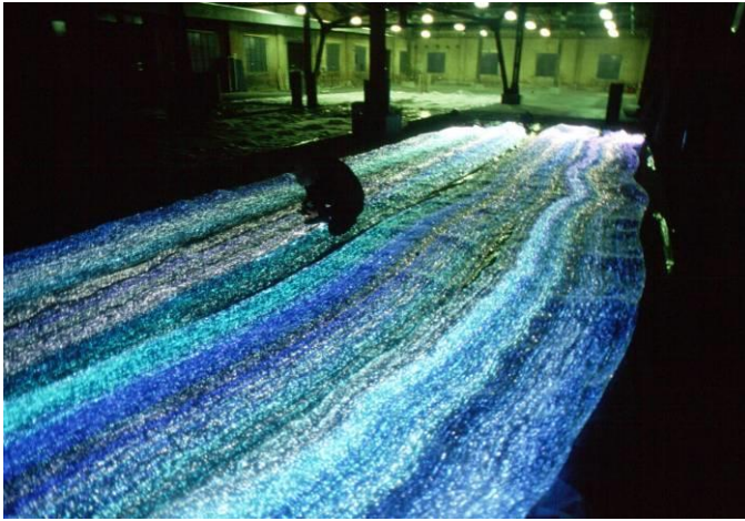
Image: light emitting cloth of woven optic fibre & stainless steel wire
